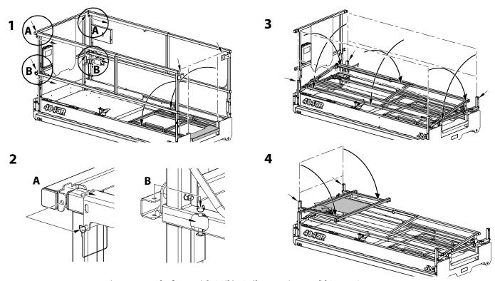
Figure 3-9. Platform with Rail in Rail Extension - Fold Down Sequence
