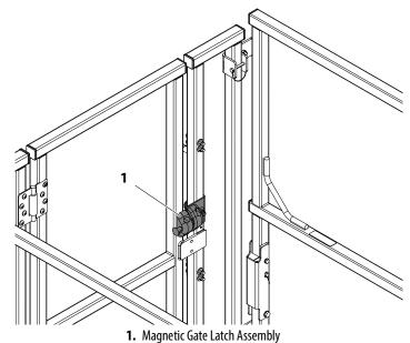
Figure 6-16. Magnetic Gate Latch Installation
