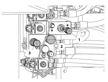
Figure 3-14. Hydraulic Brakes - Manual Disengage (Inside Right Side Compartment Door)
