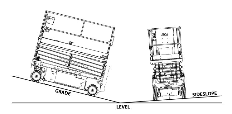
Figure 3-6. Grade and Sideslope Definition
