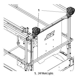
Figure 6-9. Work Lights Installation
