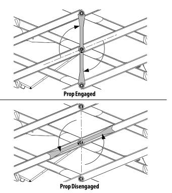
Figure 5-2. Scissor Arm - Safety Props (One each side of machine)
