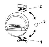
The switch should be set to the **OFF position (3)** when not using machine or parking the machine overnight.
