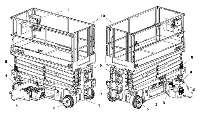
**Figure 2-1. Daily Walk-Around Inspection** (Side Compartment Doors Open)
