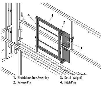
Figure 6-5. Electrician's Tree Installation
