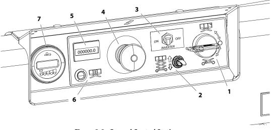
Figure 3-2. Ground Control Station
