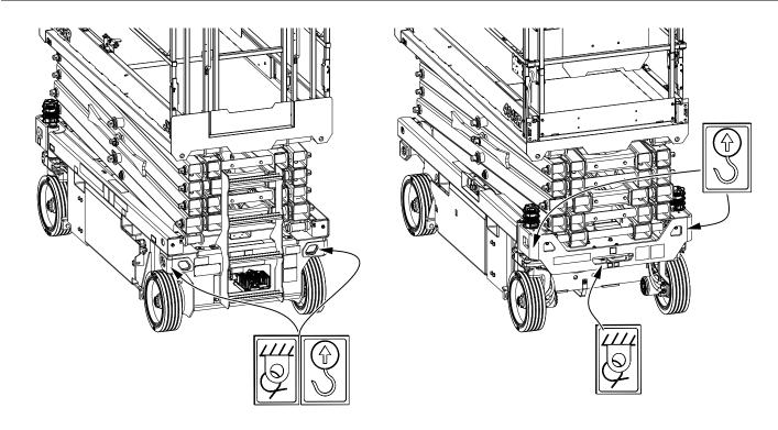
Figure 3-13. Tie Down and Lift Lug Locations
