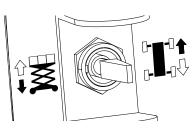
This toggle switch is used to select operation of either the drive or lift function. After selecting a function, the joystick controller must be moved in the proper direction in order to activate that function. Only change the function selected, with the joystick in the neutral position. Otherwise, the function selected will not change until the joystick is returned to the neutral position.
