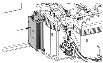
Figure 6-1. DC/AC Power Inverter
