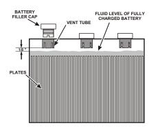
Figure 5-5. Battery Fluid Level.
